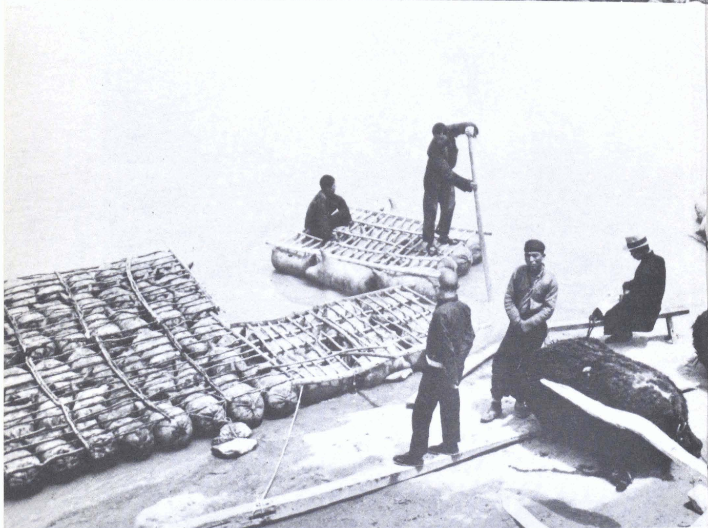
Rafts made of inflated sheepskins or oxhides, in use on the Yellow River in northwest China.
